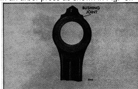
Fig. 7 - Location of Bushing Joint
