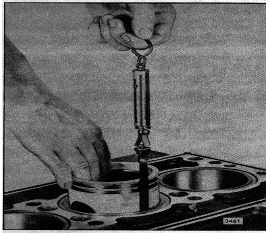
Fig. 8 - Measuring Piston-to-liner Clearance
